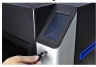
The 2018 Tiertime line of 3D printers includes a spare USB port for loading print tasks from a USB memory stick. A print task is a sliced 3D model file with print settings embedded.
